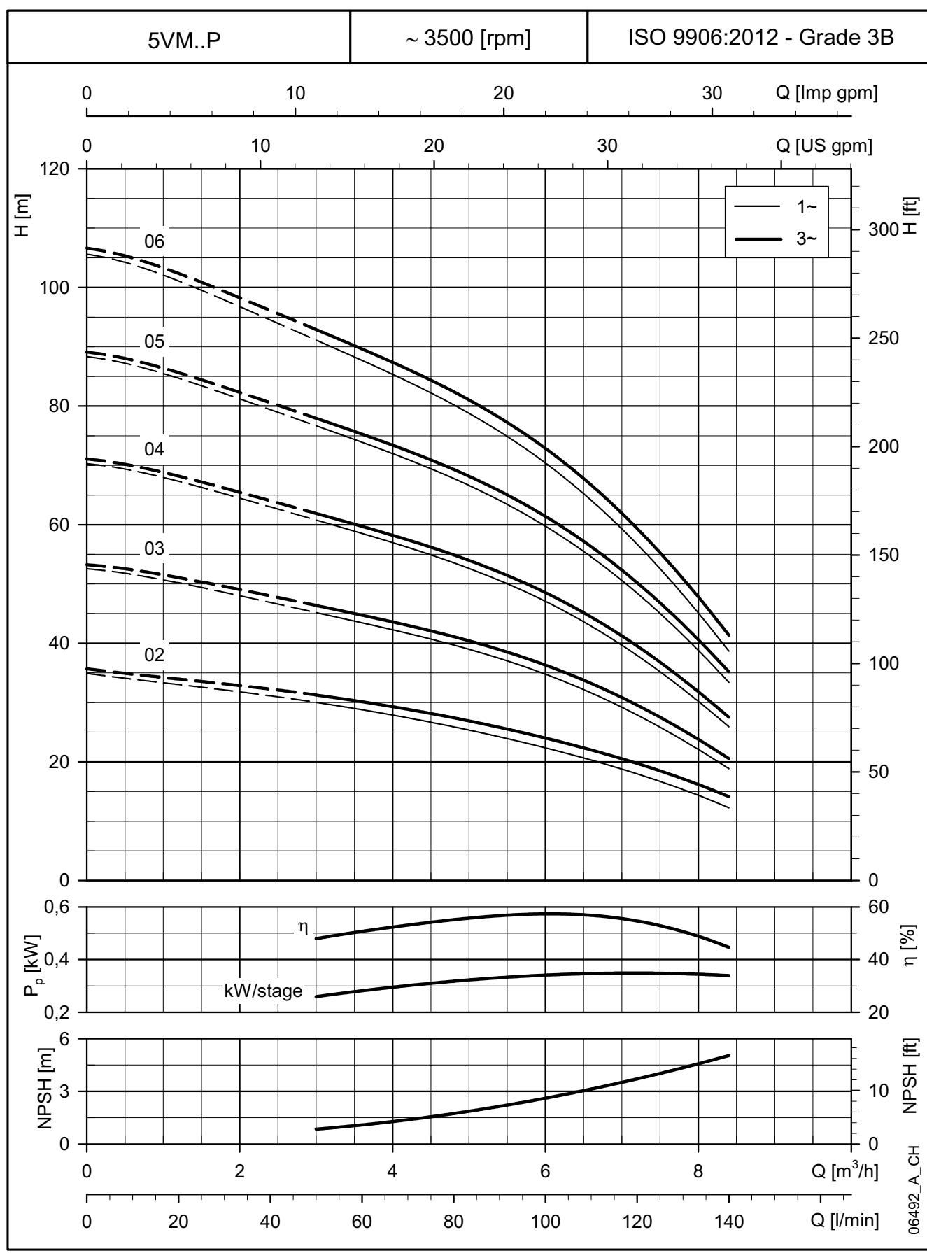
These performances are valid for liquids with density  $\rho = 1.0$  Kg/dm<sup>3</sup> and kinematic viscosity  $v = 1$  mm<sup>2</sup>/sec.
